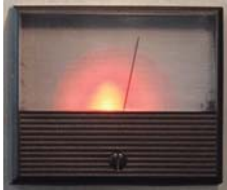
Figure 1. The galvanometer display with lit background during a run.
