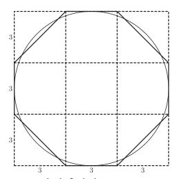
Figure 2. The Egyptian method of calculating  $\pi$ .
