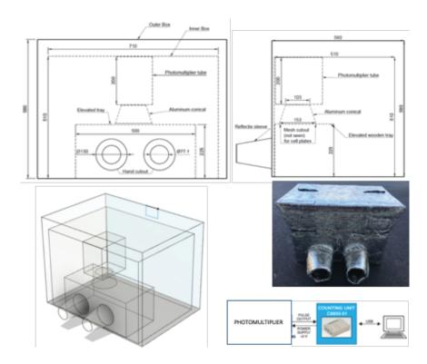
**Figure 1. Design of the light box that was tailored to measure biofield therapy from the hands of practitioners.** The practitioner placed their hands through the cutouts, within the elevated wooden tray and underneath the cell plate tray. The cells lay on the cell plate tray. The PMT box houses the PMT (not shown); the cables thread through the upper window flaps. The schematic details the connection of the PMT via the counting unit to the laptop PC. All measurements are in millimeters.
